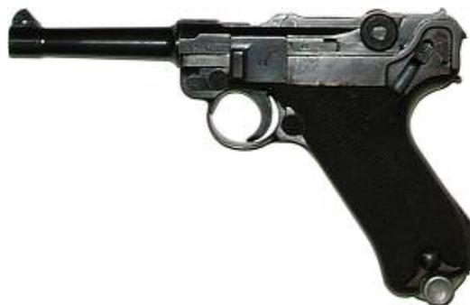
By improving on the Borchardt design, Georg Luger was able to produce a series of Self-Loading pistols known as the Parabellum pistols. Luger attempted to market his pistols to the German Army but the pistol was chambered for too light a cartridge, in their view. As a result, Luger developed the 9 x 19mm Parabellum round and altered his pistol design to accept this new cartridge. The result was a resounding success and the Luger
