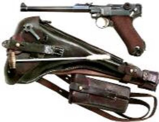
This carbine version of the Luger was issued to machine gun and Artillery detachments in 1917. It has a 7.5 inch barrel and was fitted with a detachable wooden stock and an optional 32-round 'snail' drum magazine. It became a very popular close quarter's battle weapon and it is perhaps the success of this weapon that led to the German
